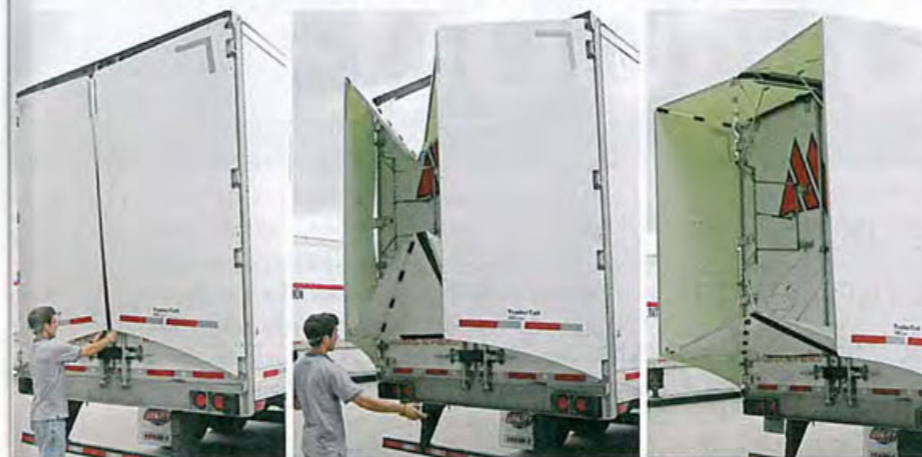
▼ Despite its size, TrailerTail weighs in at less than 80kg
