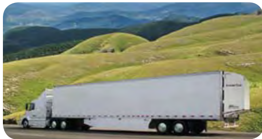
Tractor-trailer with aerodynamic drag at the rear (TrailerTail), side skirt and wheel covers Photo courtesy of ATDynamics
